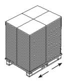
Both Sheet Directions (Width & Length) are less than 29 inches. The shipping package is 2 skids with 2 tiers of paper for a total of 4 tiers of paper. The two skids are joined together to allow them to be separated.
