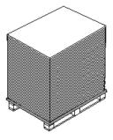
Both Sheet Directions (Width & Length) are 29 inches or greater. The shipping package is 1 skid with a single tier of paper.
